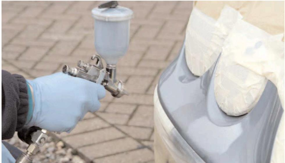
**Figure 2** Typical SMART repair
